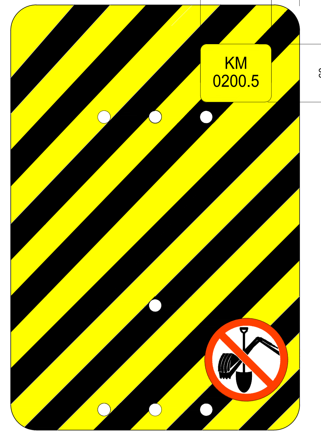
REAR OF SIGN (TYPE 2 SIGN SHOWN, TYPE 1 TO BE EXTENDED TO MATCH FRONT) (TYPICAL KP VALUE IS SHOWN)
