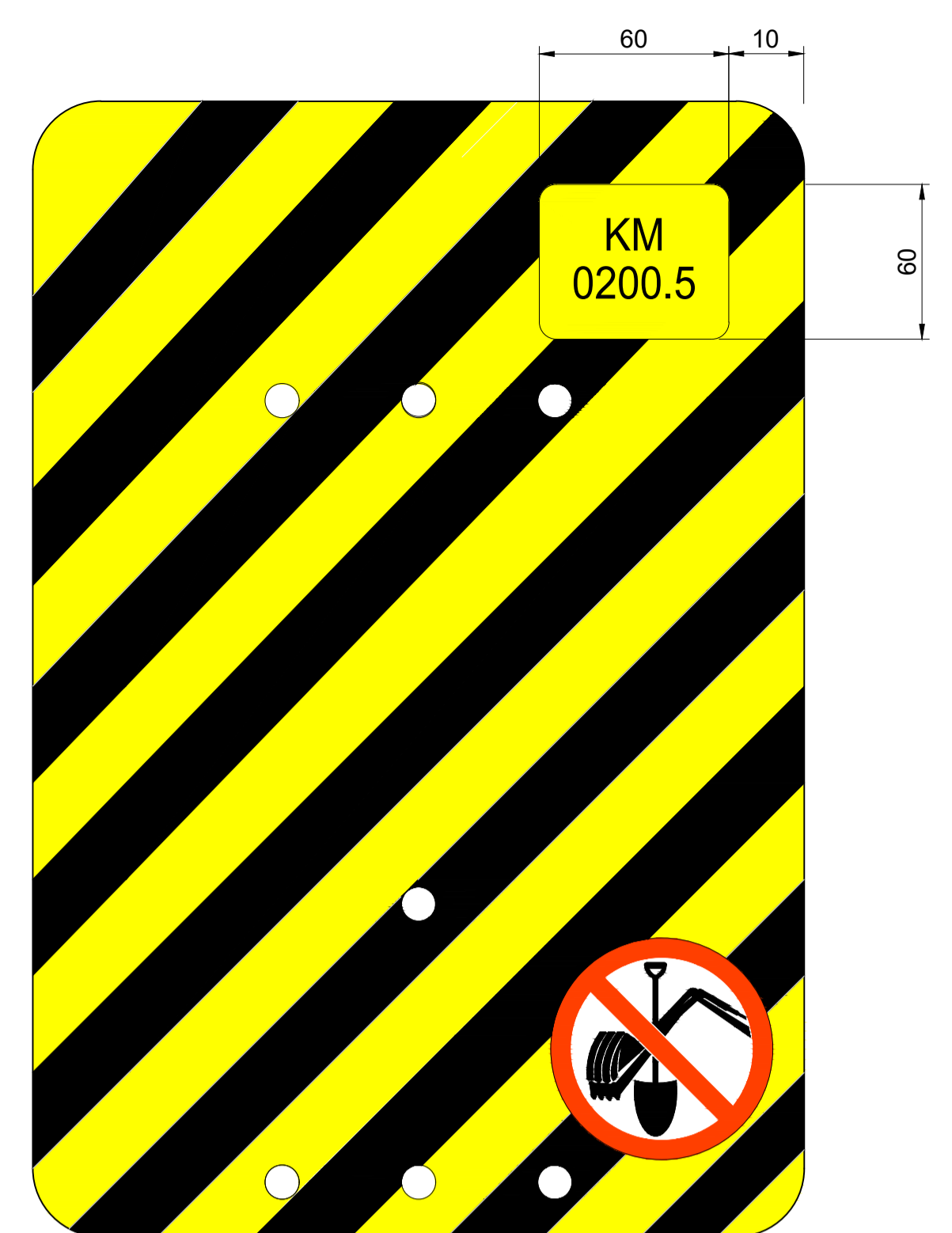
REAR OF SIGN (TYPE 1 SIGN SHOWN, TYPE 3 TO BE EXTENDED TO MATCH FRONT) (TYPICAL KP VALUE IS SHOWN)
