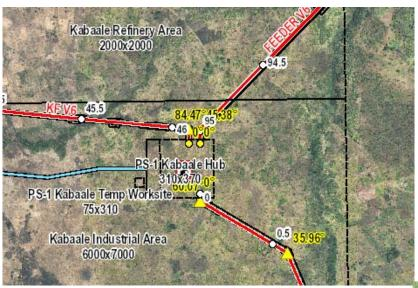
Pump Station #1 will be located at the Kabaale Hub within the area designated for the refinery. Electrical power supply will be provided from the Tilenga CPF.
