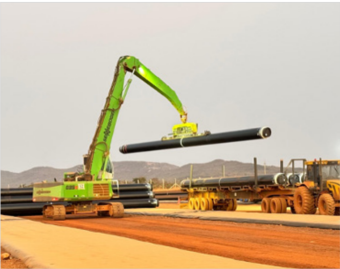
TIS yard - Ongoing PUF pipes load-out on MLC trucks to be shipped to MCPYs.
