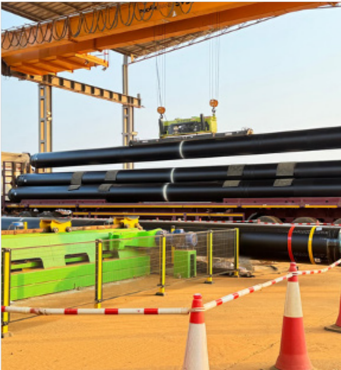
TIS Plant outgoing - PUF pipes load-out using overhead crane.
